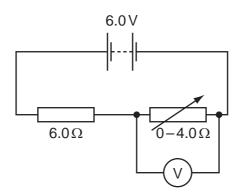
What is the range of the voltmeter reading?
