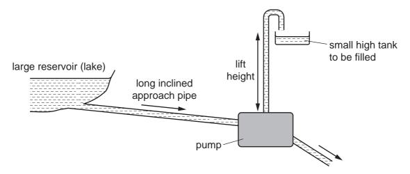
In one such pump the long approach pipe holds  $500 \, \text{kg}$  of water. A valve shuts when the speed of this water reaches  $2.0 \, \text{m s}^{-1}$  and the kinetic energy of this water is used to lift a small quantity of water by a height of  $15 \, \text{m}$ .
